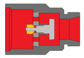
Figure 10 FE with thermal safety valve
