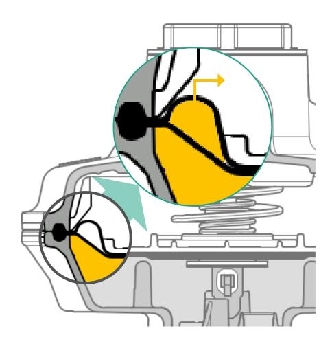
Figure 8 FE 2nd stage double diaphragms
