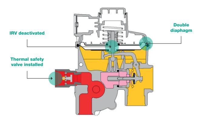
Figure 9 FE with vent limited version
