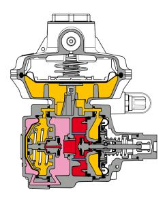
Figure 6 FE with slam shut
