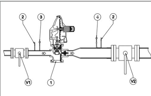
Fig. 1.1. In-line Installation
